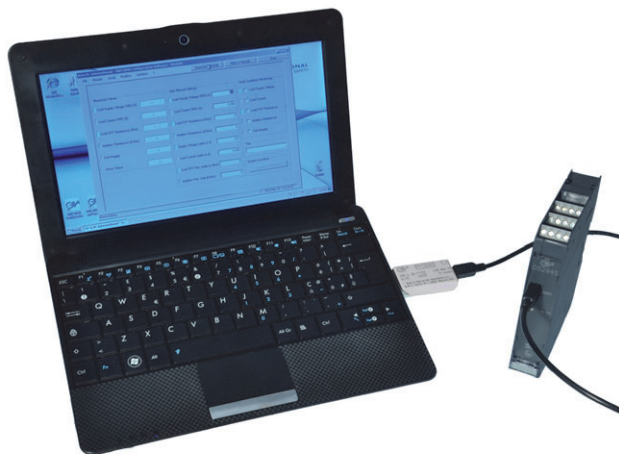
SWC5090 Software and PPC5092 USB Adapter
